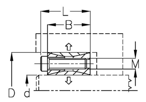
$\begin{array}{lll} \text{B mm} & = 24 \\ \text{d H8 mm} & = 48 \\ \text{D mm} & = 80 \\ \text{Fit tolerance} & = \text{Aksel k11-h11, Nav N11-H11} \\ \text{F kN torque} & = 44.6 \\ \text{L mm} & = 32 \\ \text{M mm} & = \text{M8} \\ \text{P N/mm2 surface pressure on shaft/hub} = 44 \end{array}$
